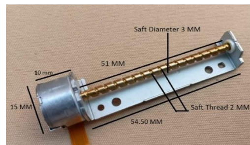
Figure 7. Four-wired stepper motor with 4.5cm shaft
