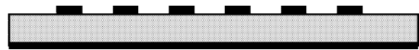
Figure 2. Cross section of the six-section lossy serpentine delay line. (line width: 20 \mu\text{m} , line spacing: 20 \mu\text{m} , line thickness: 3 \mu\text{m} , dielectric thickness : 8 \mu\text{m}/\epsilon_r=3.4 )
