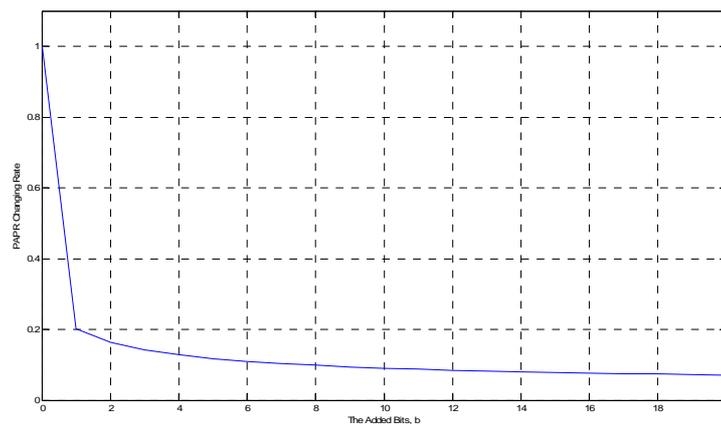
Figure 4. The PAPR changing rate in the proposed scheme
