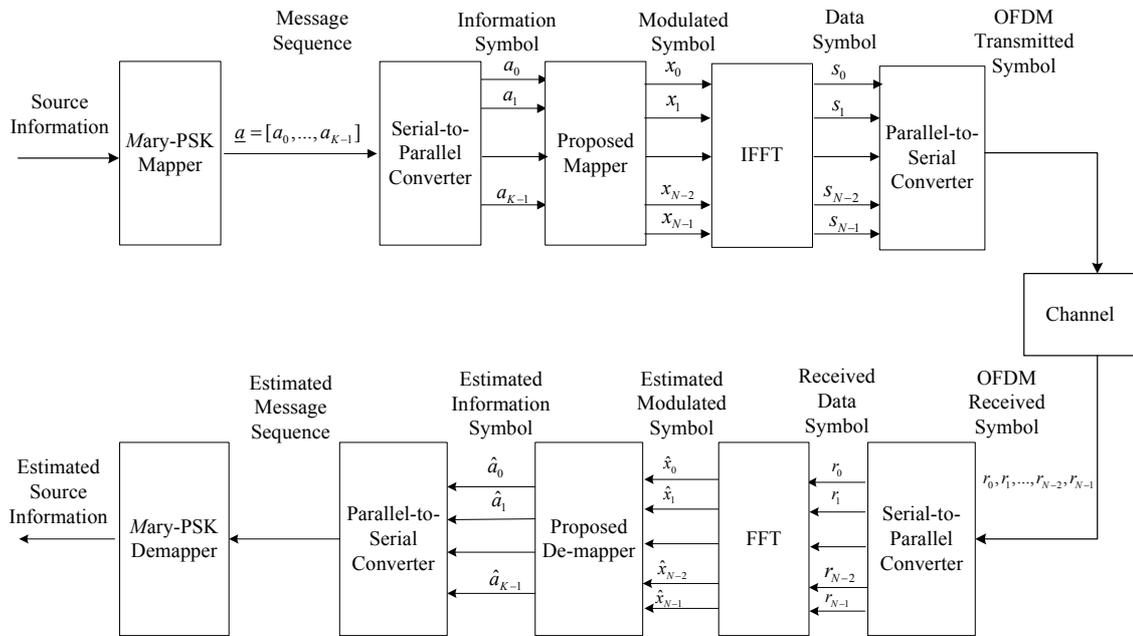
Figure 1. The block diagram of the FFT-based OFDM system
