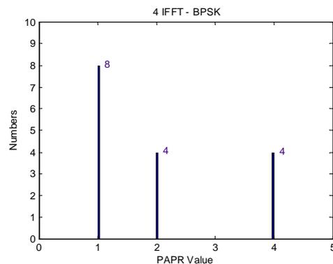
Figure 3. The histogram of PAPR in the 4-IFFT BPSK OFDM system
