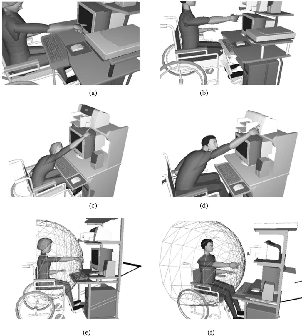
**Figure 3.** Some simulation examples: (a) 5%ile female in WS I (easy to access desk); (b) 95%ile male in WS I (hitting the keyboard tray); (c) 5%ile female in WS II (hard to operate the printer); (d) 95%ile male in WS II (reachable to the printer), and (e) and (f) the reach envelope of 5%ile and 95%ile subjects with normal upright posture in WS III, respectively.
