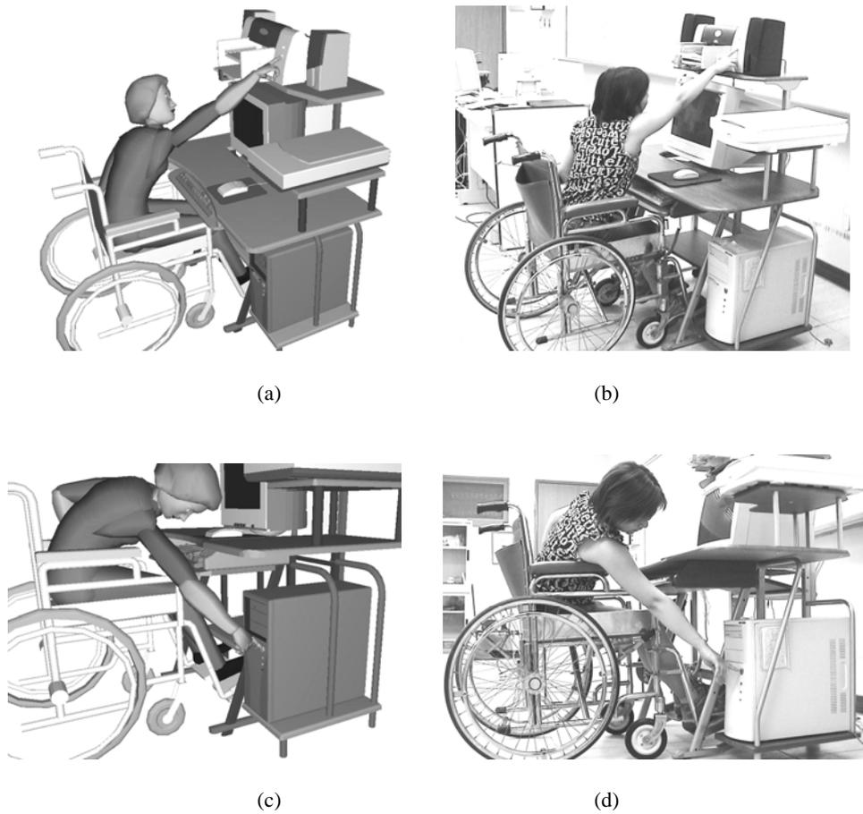
Figure 4. Comparison of simulation system and lab setup for WS I: (a) and (b) reach of printer, (c) and (d) turning the CPU system unit on and off
