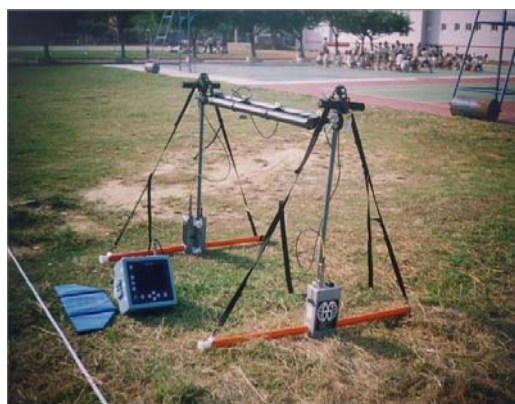
Figure 3. SIR-2 machine and 16-80MHz antenna
