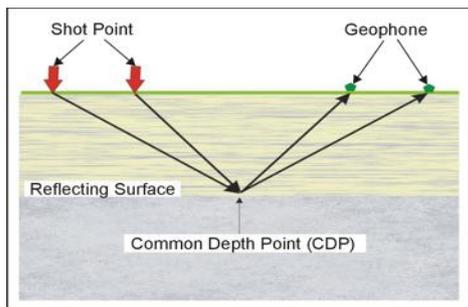
**Figure 5:** Principle of CDP test
