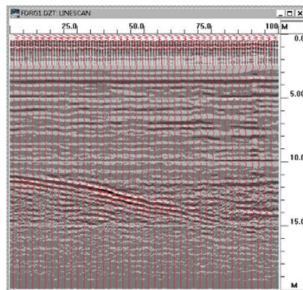
Figure 20: Overlaid demonstration of diagram and Wiggle diagram after de-convolution
