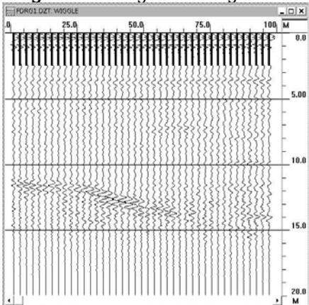
Figure 15: Wiggle diagram after gain
