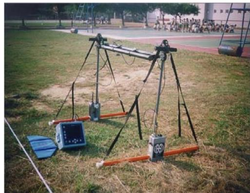
Figure 3. GSSI SIR-2 machine and 16~80 MHz antenna
