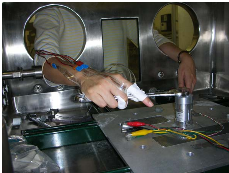
Figure 2. Wrench task simulation inside a typical glovebox (the subject did not wear glove to show the FSRs connection).
