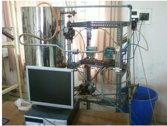
Figure 5b. Photographic view of the integrating tank experimental setup.
