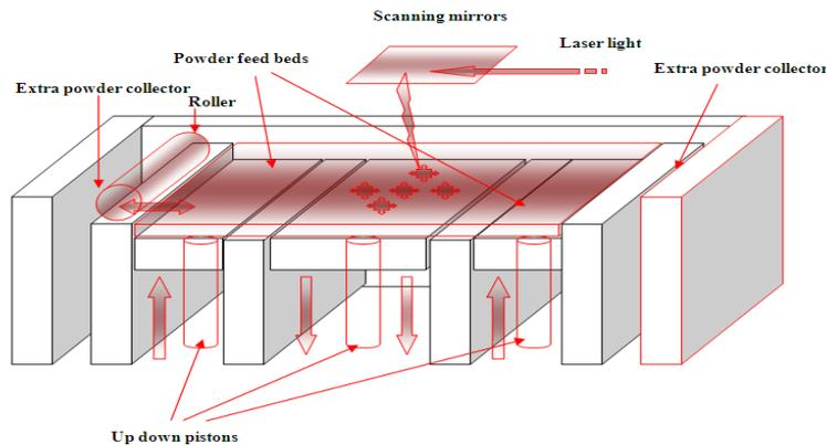
Figure 1. Block diagram of Selective laser Sintering (SLS) process [2]
