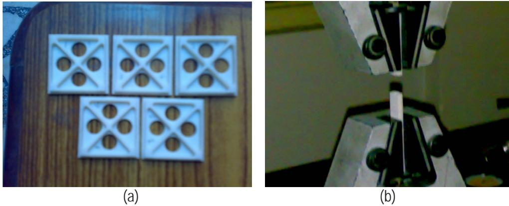
Figure 3. (a) Photograph of different specimens to measure S%, (b) Photograph of universal testing machine with sample
