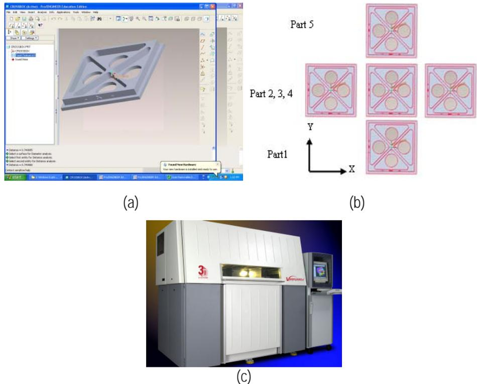
Figure 2. (a) CAD model of specimen used to study, (b) Layout of different parts placed in machine bed, (c) SLS setup used for fabrication of parts
