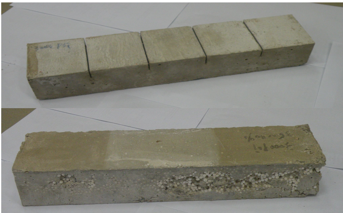
Figure 4. Concrete specimens with defects used for the dynamic plunking test
