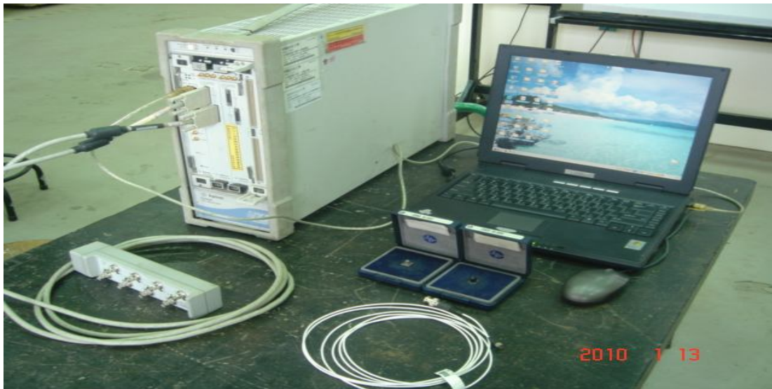
Figure 3. VXI multiple channel data acquisition system
