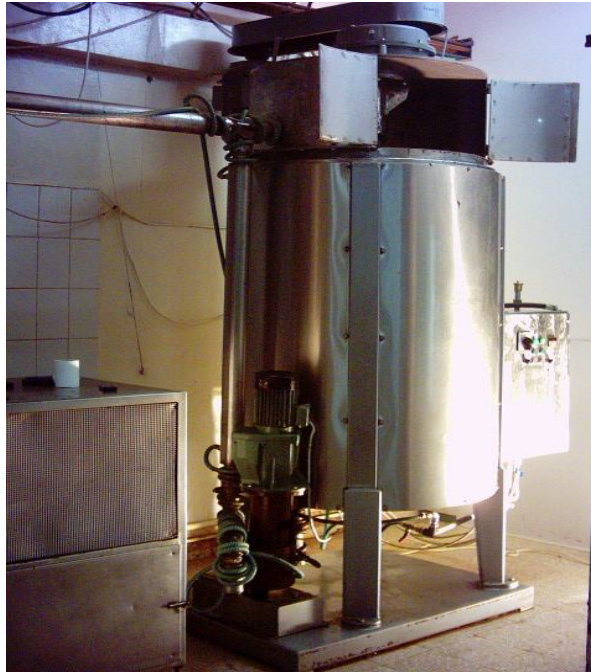
Figure 9. Newly designed machine (wiener of 1000 kg)
