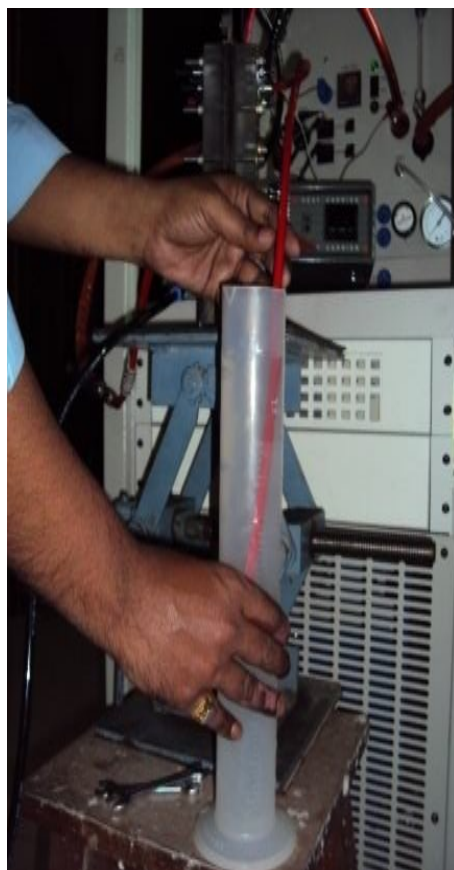
Figure 3. Photograph of experimental set up of single cell to create backpressure
