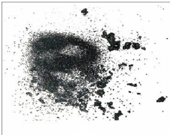
Figure 2. General megascopic view of ilmenite mineral grains after microwave heating on oxidized ilmenite with coke carbon
