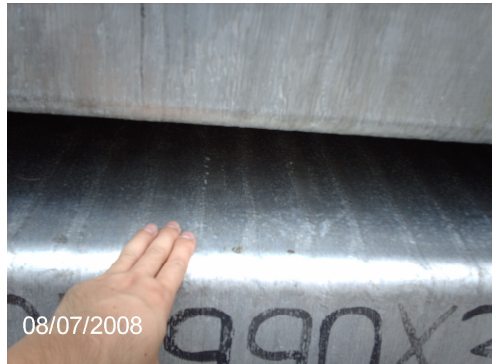
Figure 10. Laps which has the pitch of span of three fingers
