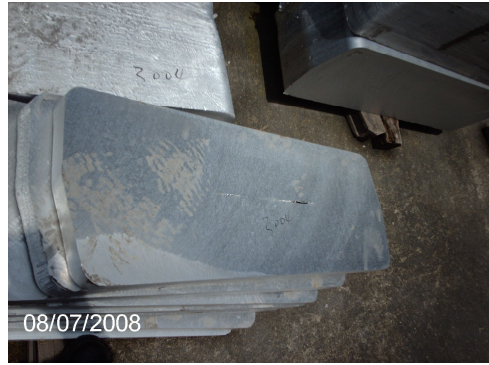
Figure 9. Liquation inside of ingot
