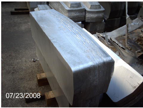
Figure 8. Cold shut on the bottom sides
