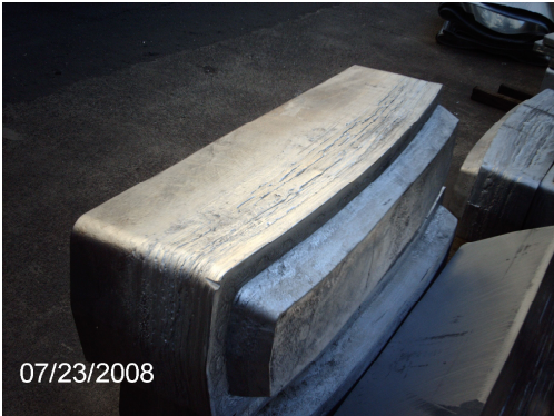
Figure 5. The breed-out in the bottom of ingot
