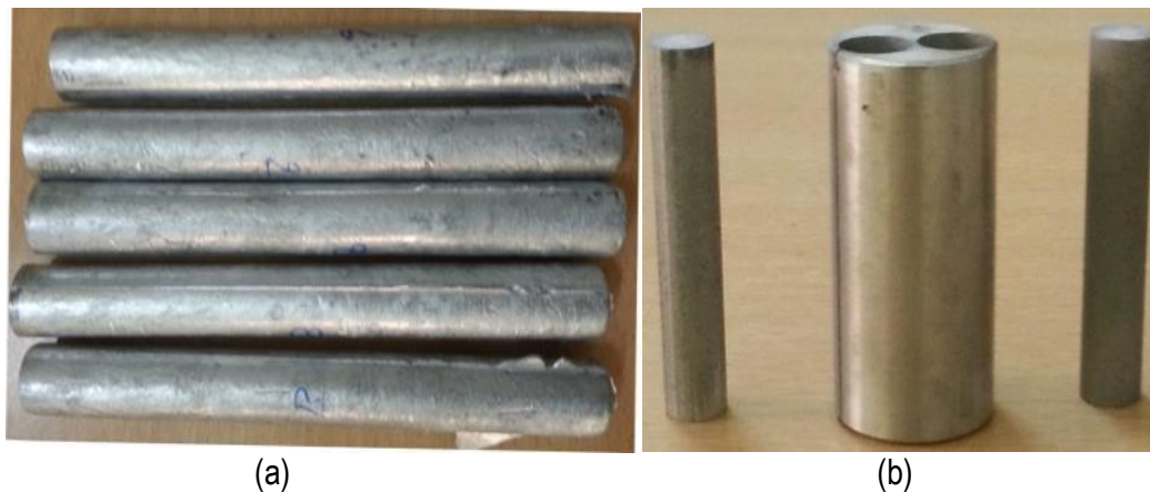
Figure 1. Specimens of composite (a) cast (b) wear
