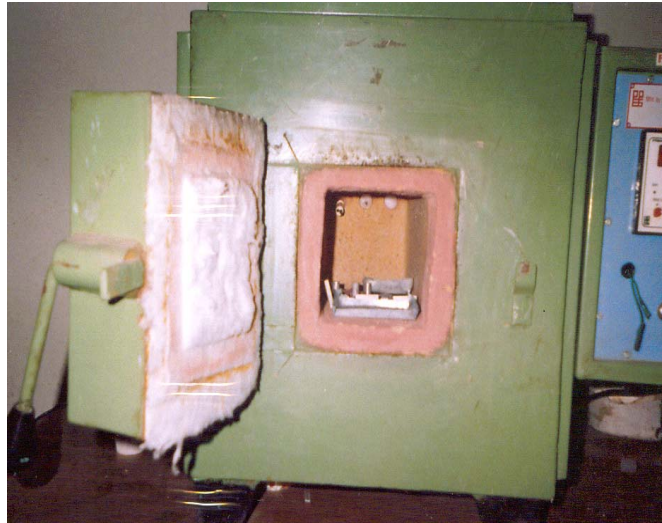
Figure 1. Photograph of muffle furnace used for heat treatment.
