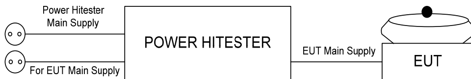
Figure 3. Power consumption measurement set up.
