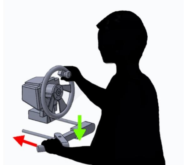
**Fig. 1.** Refitted manual controller (red arrow/pushing forward corresponded with acceleration, whereas green arrow/pushing down corresponded with braking)
