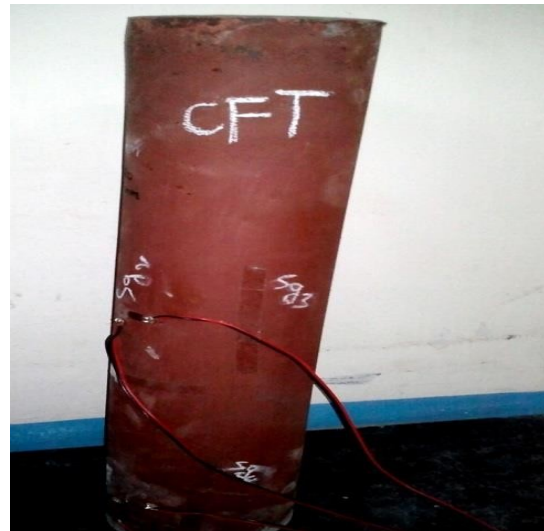
(b) Failed CFT specimen
