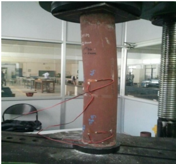
(a) Tested CFT specimen
