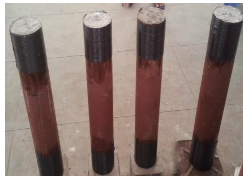
(b) CFRP wrapped specimens
