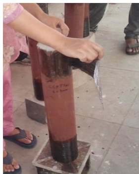
(a) Wrapping of CFRP 1 layer
