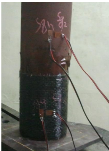
(a) Tested CFT specimen
