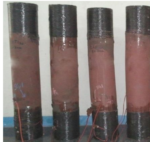
(b) Failed CCFT specimens
