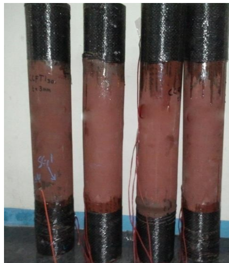
(b) Failed CCFT specimens
