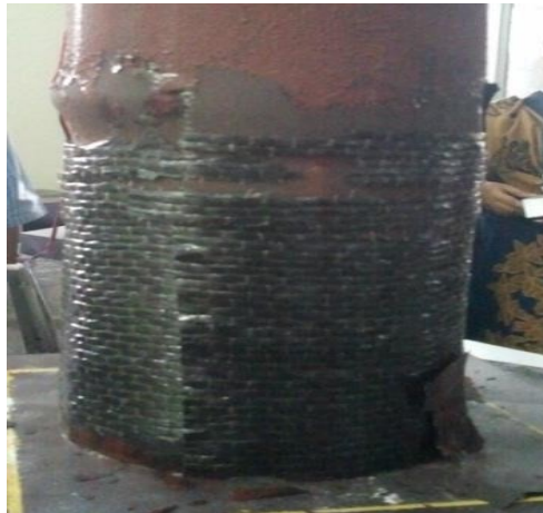
(a) Tested CFT specimen
