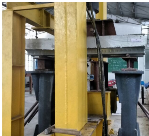
(b) Photo of a flexure load test of a composite slab
