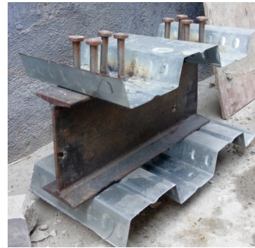
Fig. 6. Push-out test specimen
