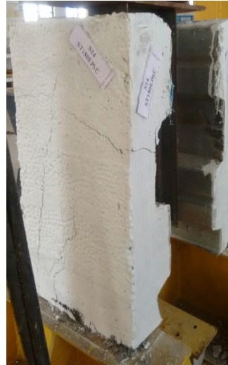
Fig. 25. Crack pattern in slab 'PET1'
