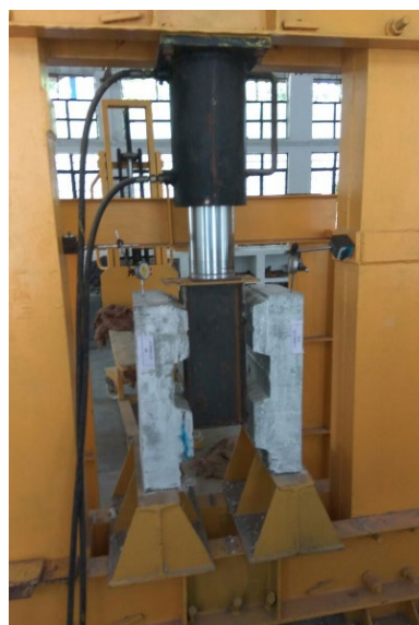
(b) Photo of a push-out test of composite slab in progress
