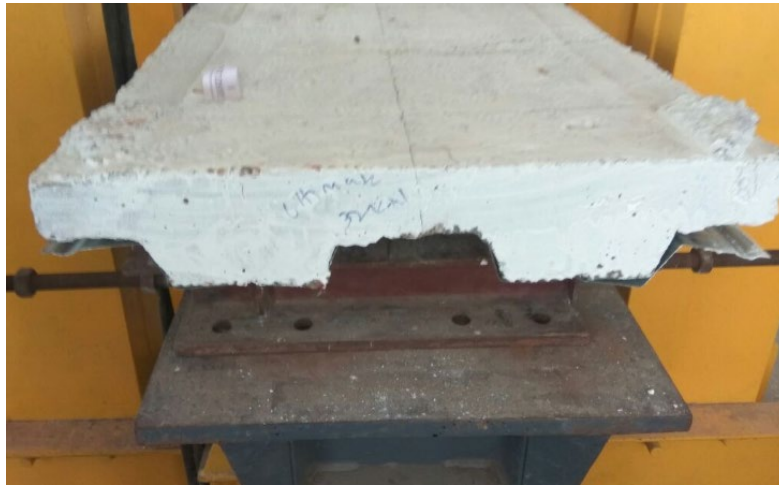
Fig. 20. Slip of steel sheet in FET2SS2 composite slab
