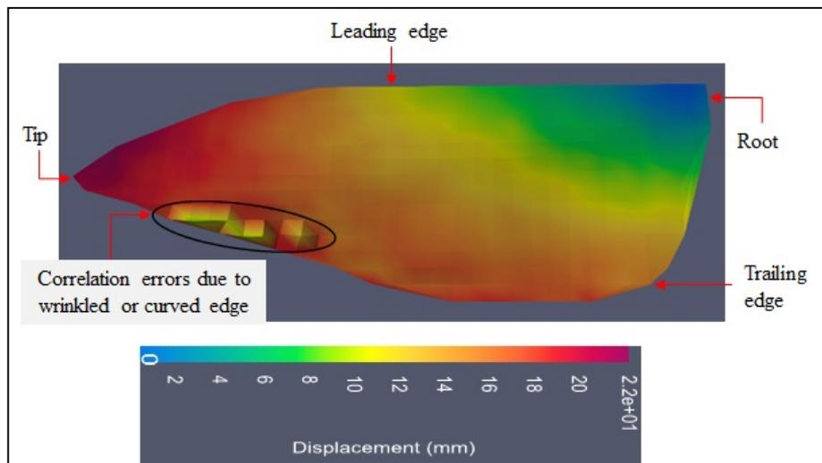
Fig. 13. Wing deforming shape measured using 3D-DIC, at the end of upstroke
