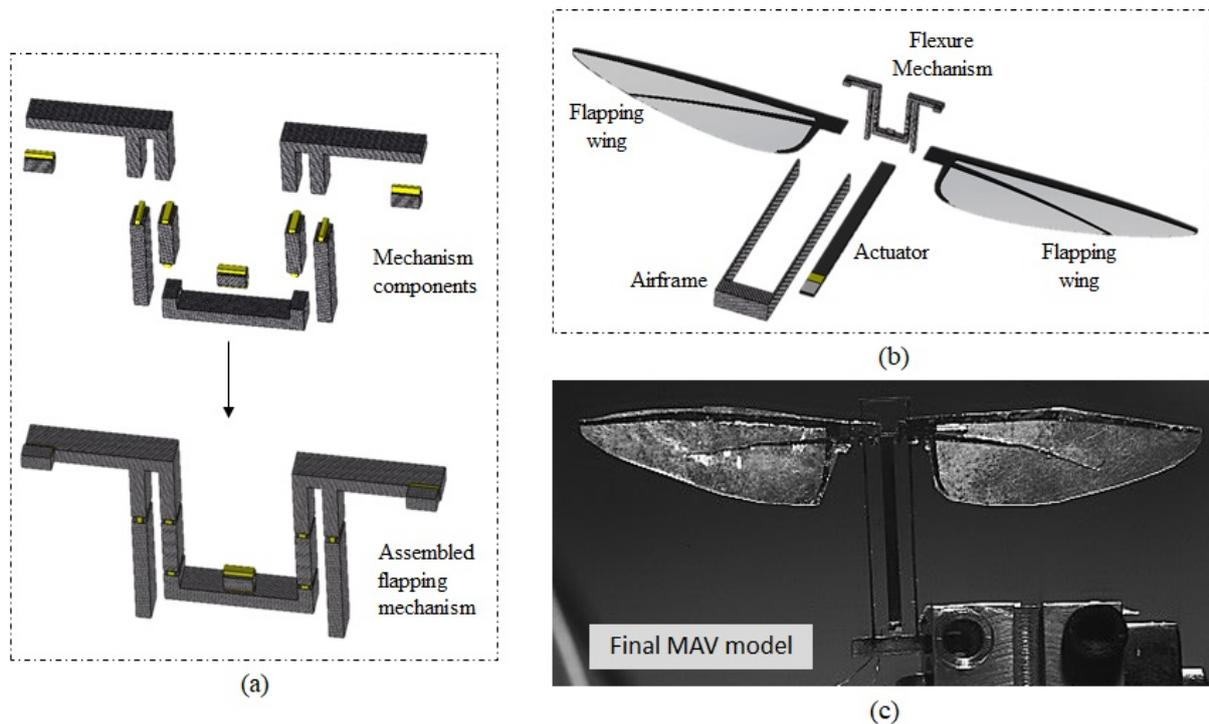
**Fig. 11.** Development process for the MAV model, (a) Assembly of the compliant mechanism (b) Assembly of the MAV model (c) Fabricated two-winged insect-inspired MAV model
