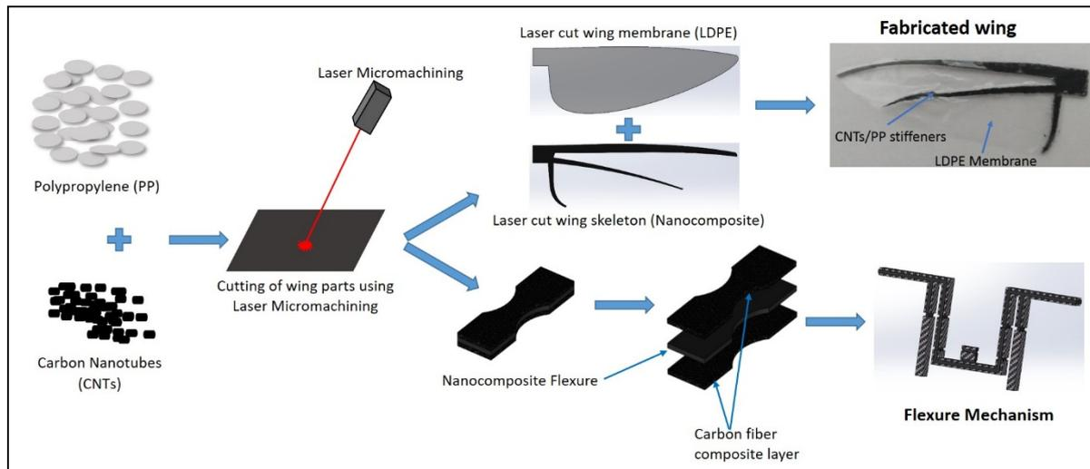
Fig. 10. Manufacturing process for wing and mechanism
