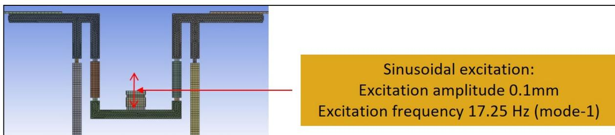
Fig. 8. Wing-mechanism design under resonance excitation
