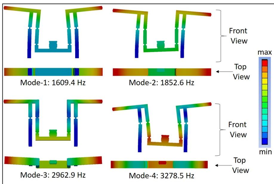
Fig. 5. Modal analysis results for flapping mechanism
