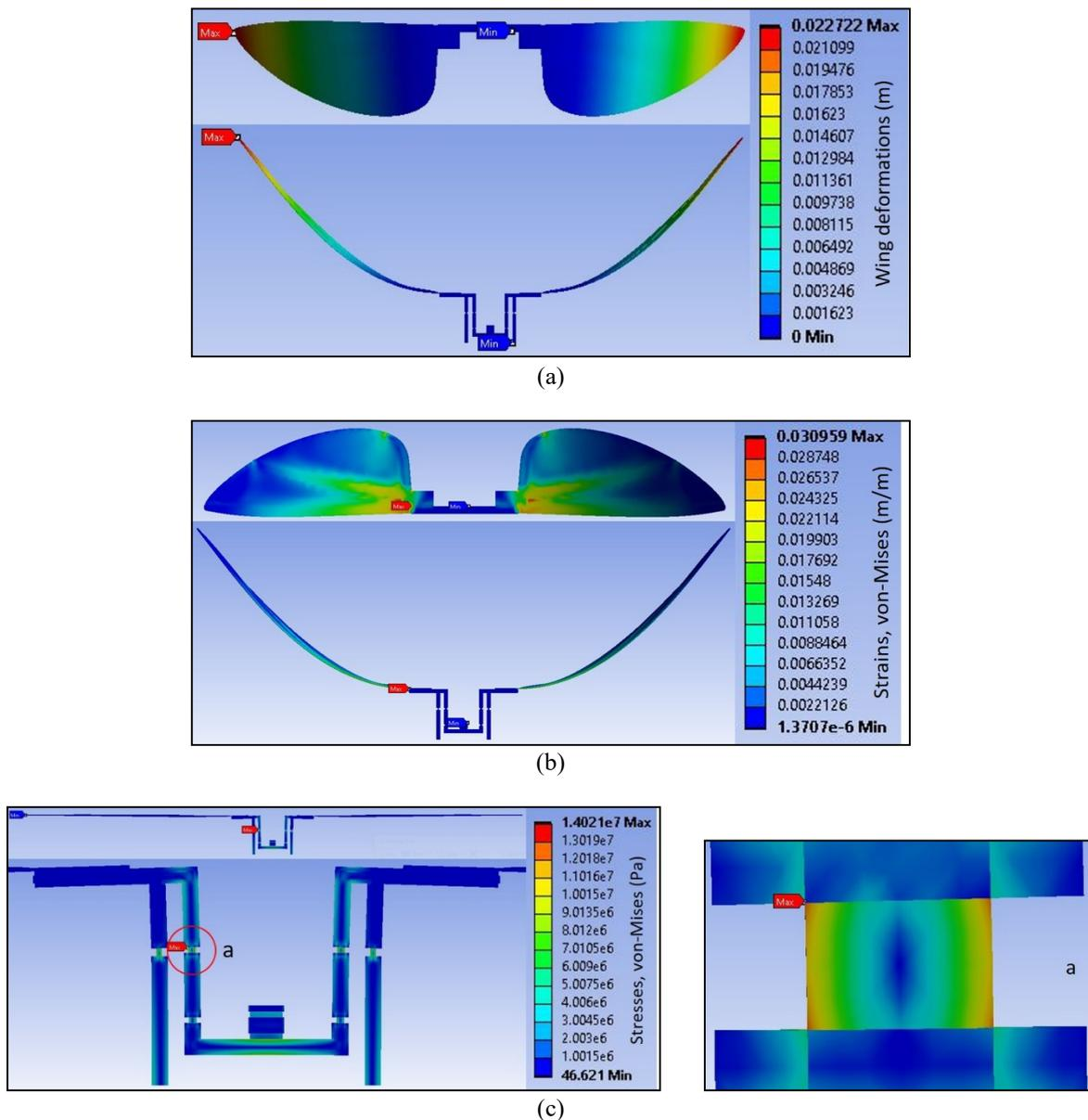
Fig. 9. Computational structural dynamic study results for combined wing-mechanism model (a) wing deflections (b) strains distribution (c) stress distribution
