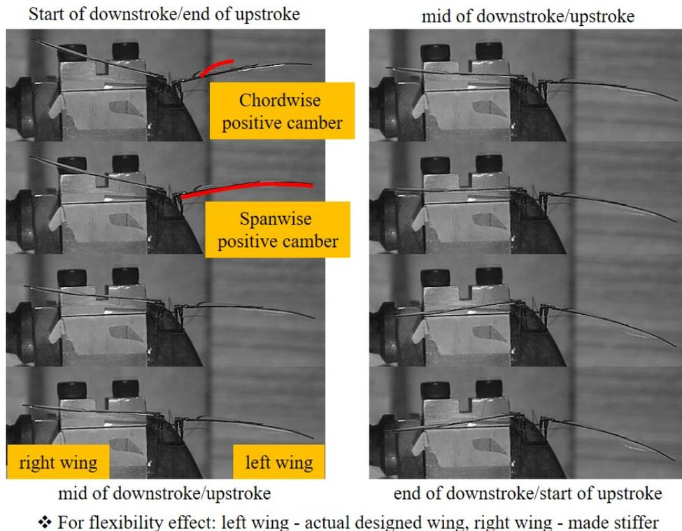
**Fig. 14.** Wing motion recorded using a high-speed camera at 1000fps. Left side of the image shows start to mid of the flapping stroke, Right side of the image shows mid to end of the flapping stroke
