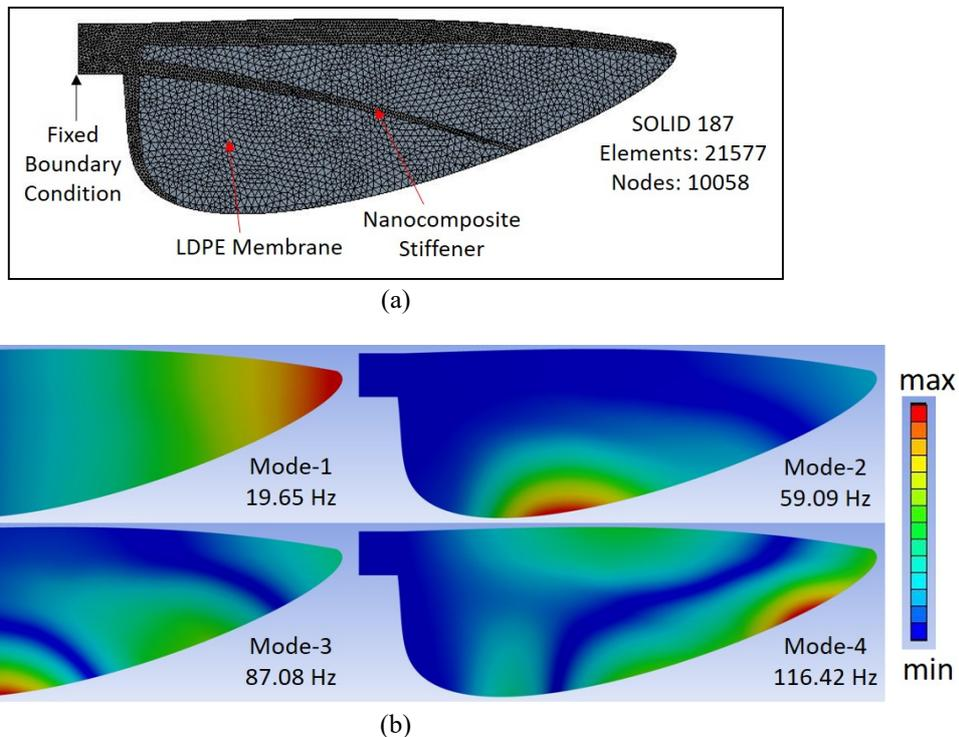
Fig. 3. (a) Mesh details and boundary conditions (b) Modal analysis results for the wing
