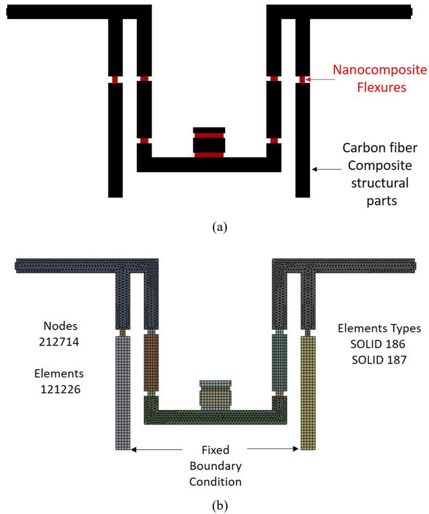
Fig. 4. Mechanism model used for modal analysis (a) mechanism components and corresponding materials (b) mesh details and boundary conditions
