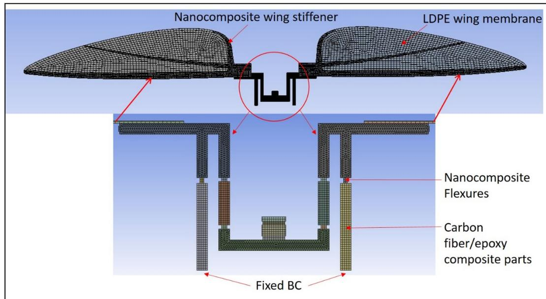
**Fig. 6.** The mechanism-wing design under structural dynamic analysis
