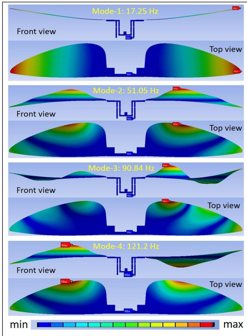
Fig. 7. Four fundamental modes for the combined wing-mechanism model
