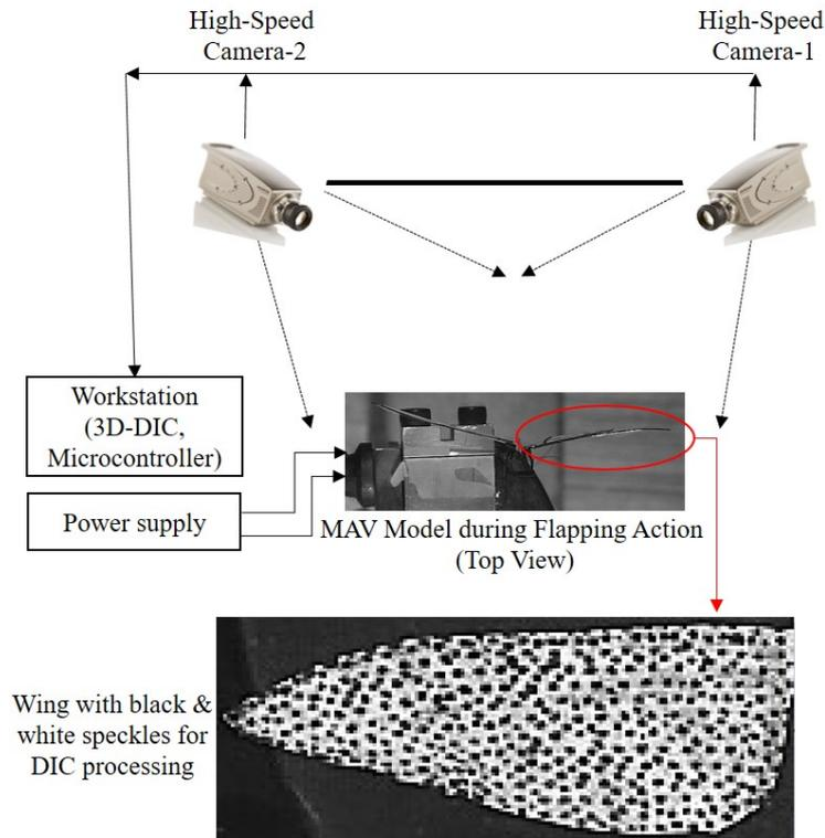
Fig. 12. In-house 3D-DIC setup for experimental structural dynamic testing of MAV wings
