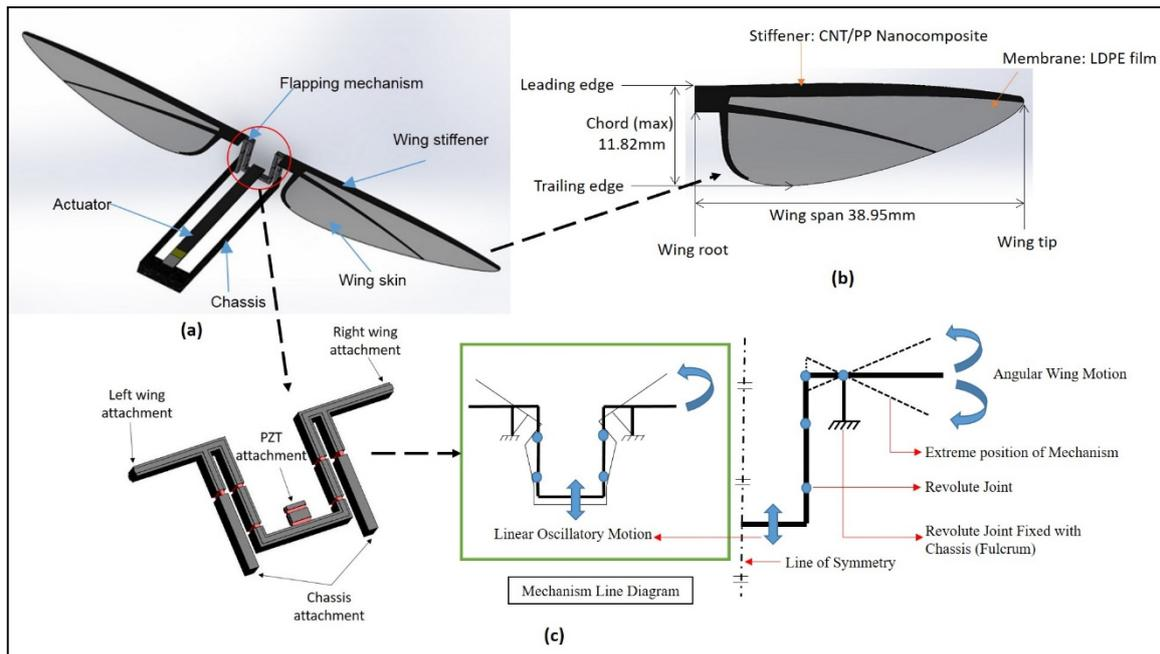
Fig. 2. Bioinspired designs, (a) MAV model (b) Flapping wing (c) Flapping mechanism
