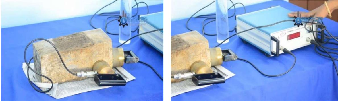
**Fig. 3.** Ultrasonic pulse velocity test setup for the brick specimen
