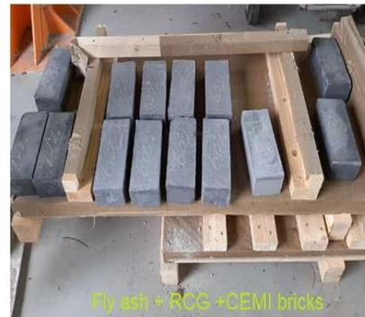
**Fig. 2.** Showing fired bricks and non-fired bricks retrieved from the molds
