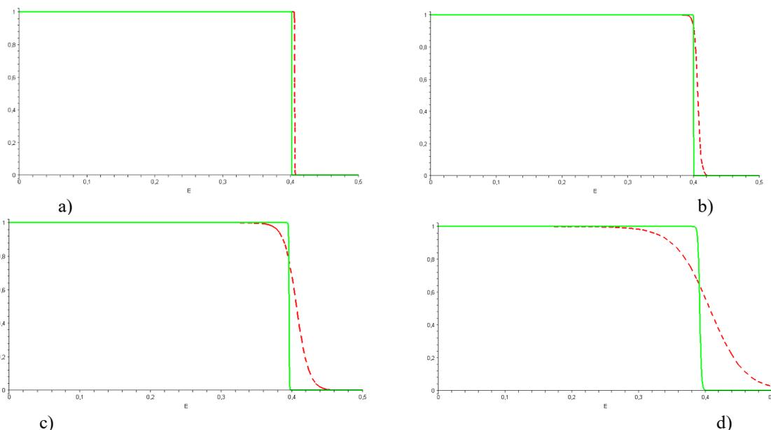
**Fig.3.** Distribution of the Fermi-Dirac function in nanoscale semiconductors at high temperatures and weak magnetic fields. Calculated by Equation (20). Solid green lines for  $H \neq 0$ , dashed red lines for  $H = 0$ . a)  $T=5$  K. b)  $T=30$  K. c)  $T=100$  K. d)  $T=300$  K
