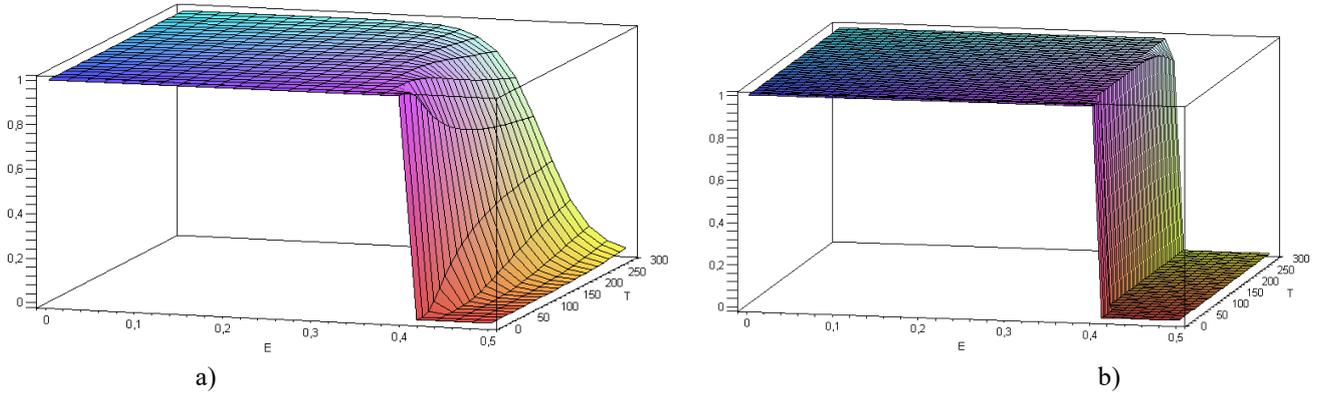
**Fig.4.** Distribution of the Fermi-Dirac function for nanoscale semiconductors in three-dimensional space at a constant magnetic field ( $H=8$  T). Calculated by Equation (20)
