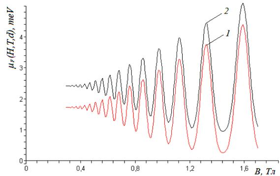
**Fig.2.** Influence of the thickness of the quantum well on the oscillations of the Fermi energy in a quantizing magnetic field. Here,  $T=4.2\text{ K}$  is calculated by Equation (18) for *InAs/GaSb/AlSb* quantum wells. 1)  $d = 8\text{ nm}$ , 2)  $d = 5\text{ nm}$
