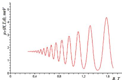
**Fig.1.** Dependence of the Fermi energy oscillations on the quantizing magnetic field for *InAs / GaSb / AlSb* quantum wells at  $T=4.2\text{ K}$ ,  $d=8\text{ nm}$ . Calculated by Equation (18)
