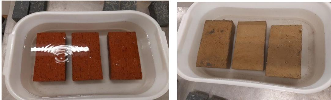
**Fig. 3.** Durability test setup for clay and PW-bricks
