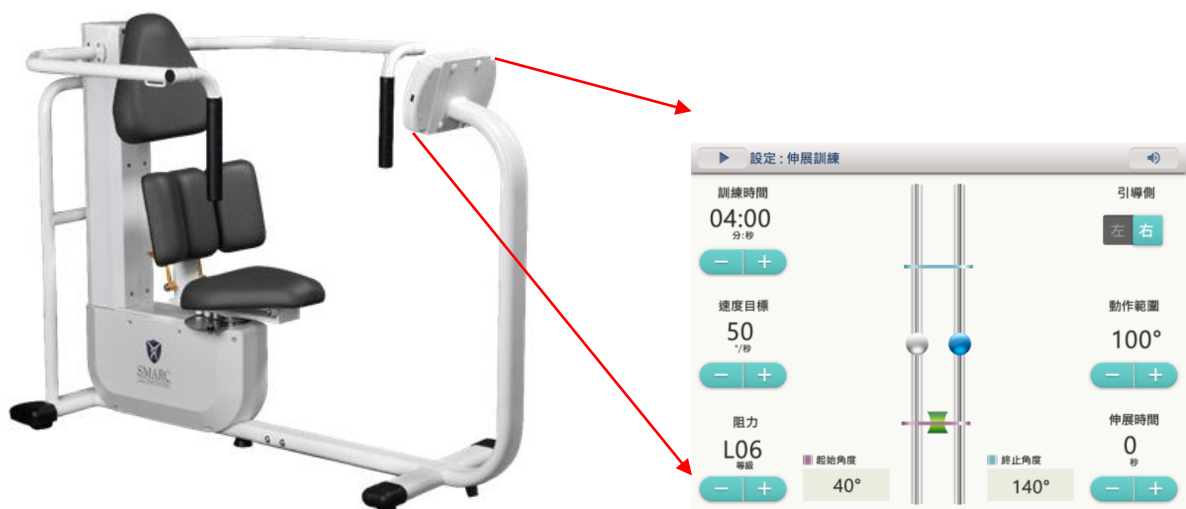
Fig. 1. A laboratory-owned shoulder-upper extremity fitness training equipment with parameters adjusting screen for stretching exercise
