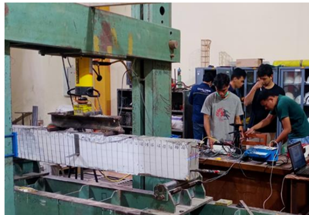
Fig. 4. Setup of beam testing
