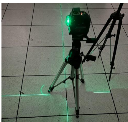
Fig. 2. Laser angle aligner consisted of a laser level meter and a tripod
