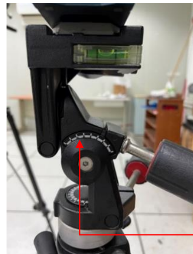
Fig. 3. Each increment is 15 degrees with adjustment range in -30 to 90 degrees.
