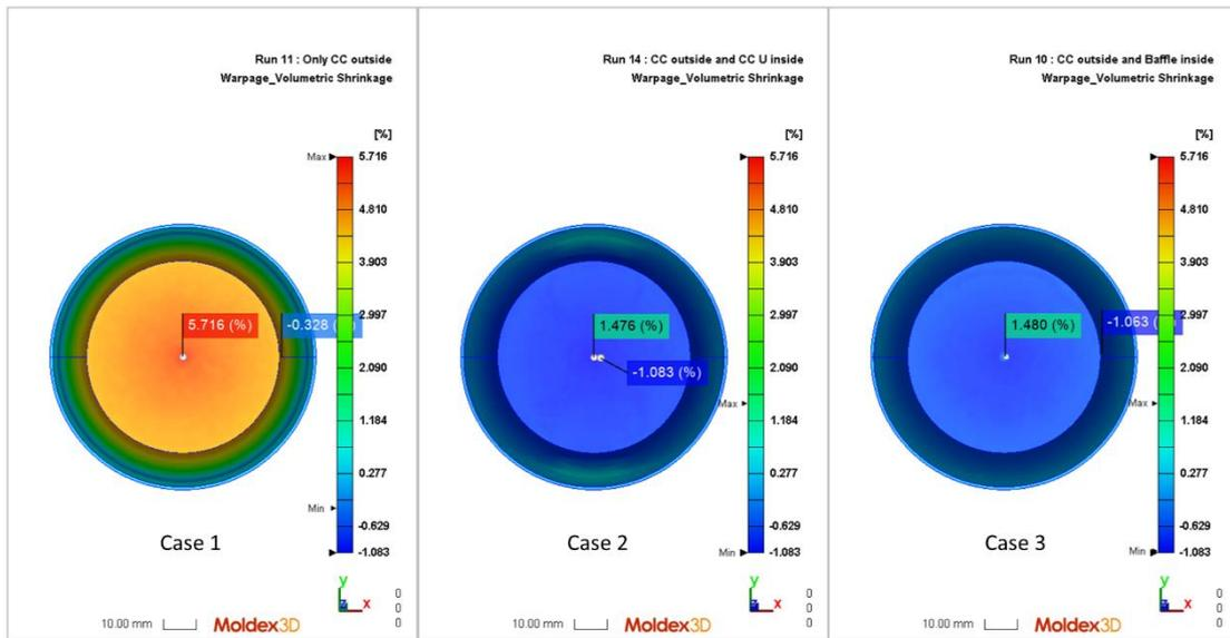
Fig. 7. The effect of cooling design on the volumetric shrinkage
