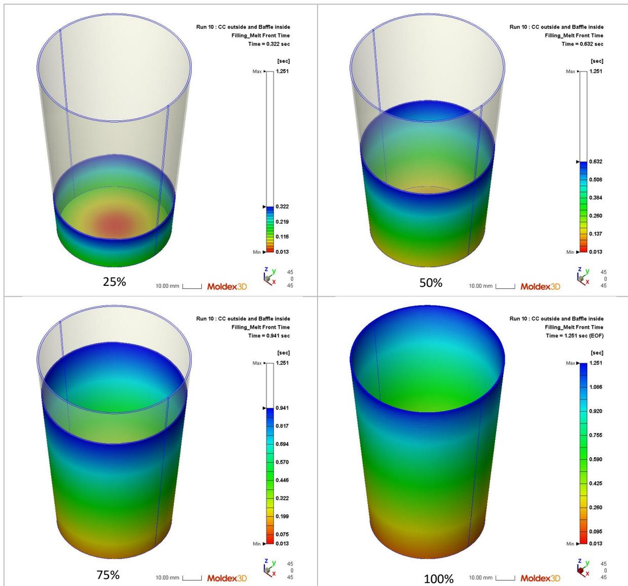
Fig. 3. Melt front time for the filling process at different stages: 25%, 50%, 75%, and 100%
