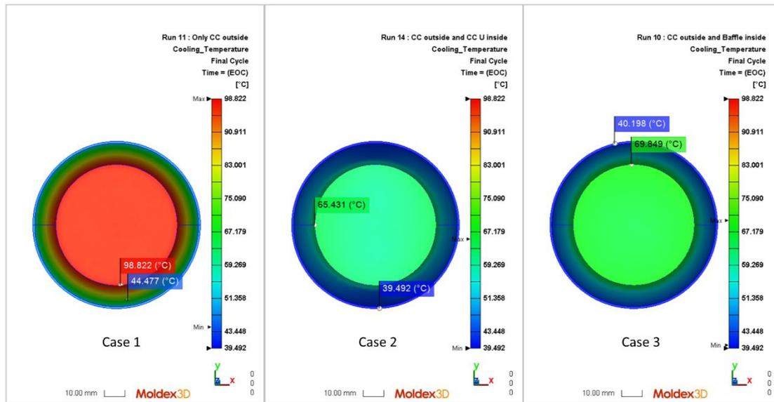
Fig. 4. Temperature distribution of the part after cooling in each of the three cases
