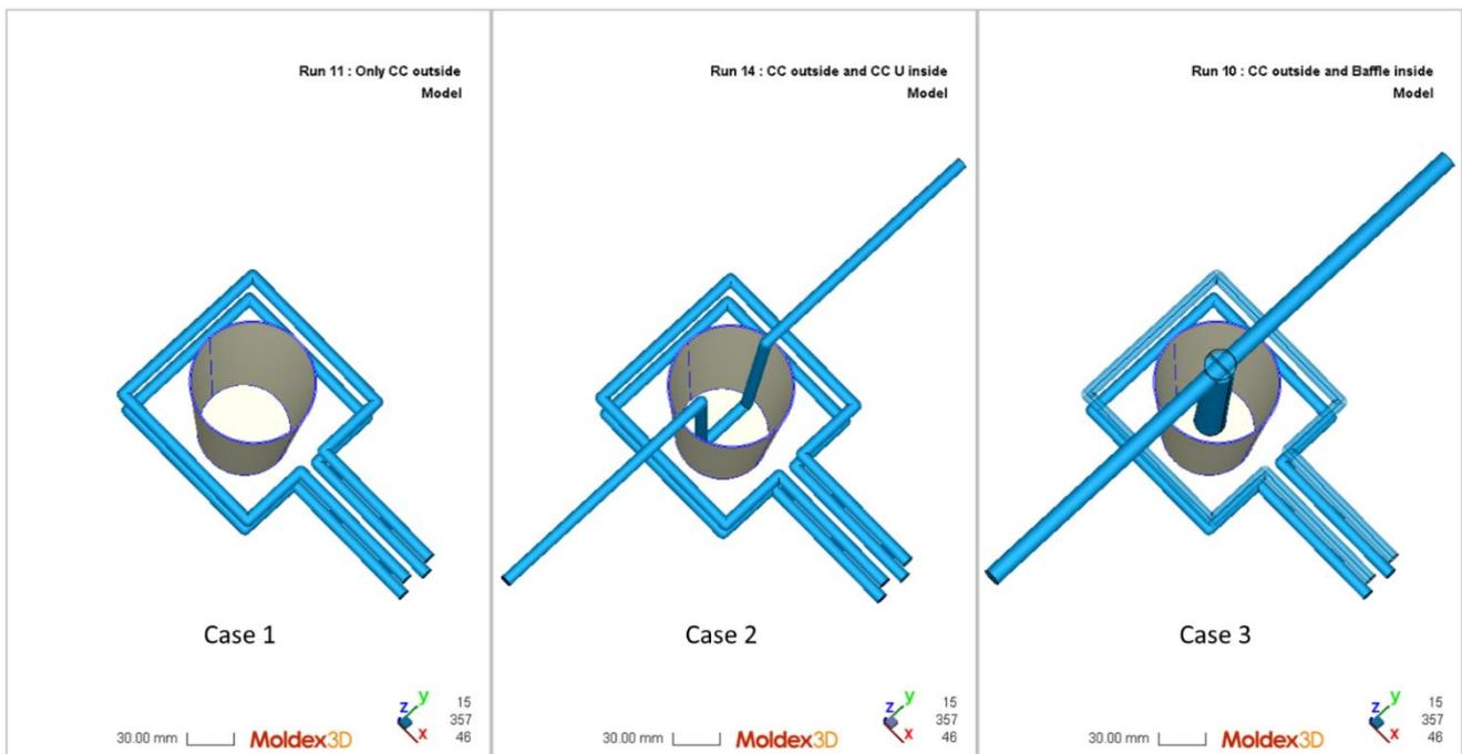
Fig. 2. Three different cooling channel designs
