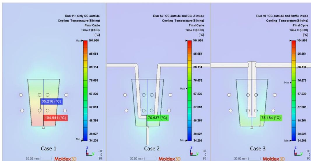
Fig. 5. Maximum cooling temperature (slicing) of the three cases
