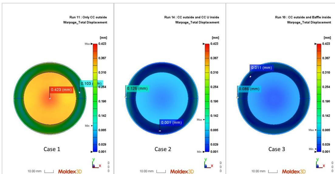
Fig. 6. Total displacement warpage of the part for the three cases with a scale factor of 10
