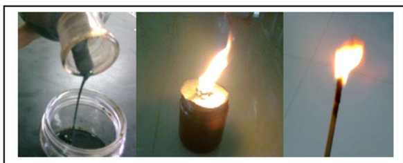
Fig. 7. Pyrolysis oil flammability test
