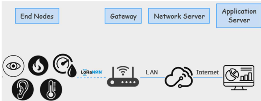
Fig. 1. Proposed LoRaWAN system architecture
