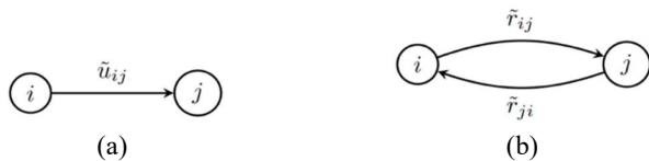
Fig. 2. (a) Arc capacities of fuzzy network. (b) Residual arc capacities.
