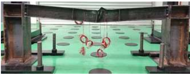
Fig. 4. Condition of pipe support with stiffener reinforcement after testing
